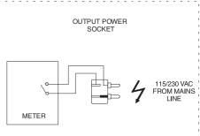
The meter works as a normally open switch. When alarm is active (MEAS > SETPOINT) the "switch" is closed.
